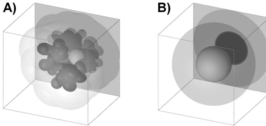
Figure 8. The geometries used for the light scattering simulations: A) The soot particle composed of three materials, namely black carbon, sulfate, organic acid. B) The sphere of equivalent volume.
