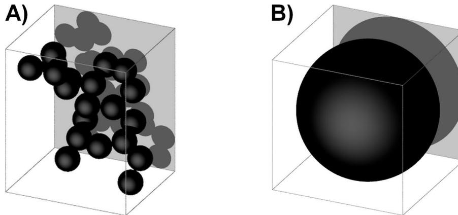
Figure 2. The geometries used for the light scattering simulations: A) The fractal-like aggregate composed of black carbon particles, B) The sphere of equivalent volume.
