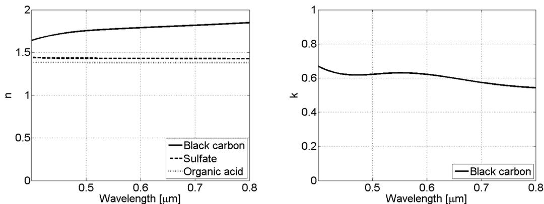
Figure 1. Complex refractive indices  $m$  used in the study, namely: black carbon  $m_c$ ,<sup>10</sup> sulfate  $m_s$ ,<sup>11</sup> organic acid  $m_a$ .<sup>9</sup>
