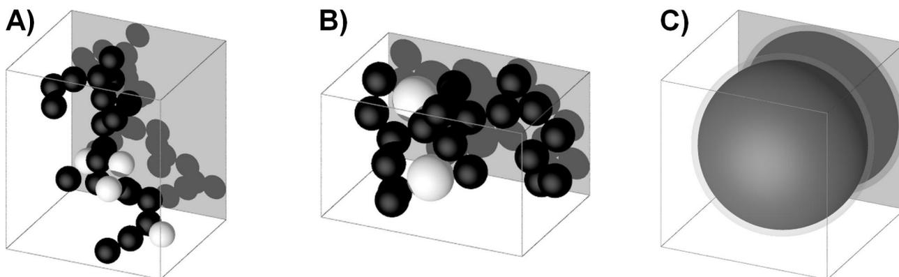
Figure 4. The geometries used for the light scattering simulations: A) The core black carbon aggregate with five spherical sulfate particles. B) The core black carbon aggregate with two ellipsoidal sulfate particles. C) The sphere of equivalent volume.
