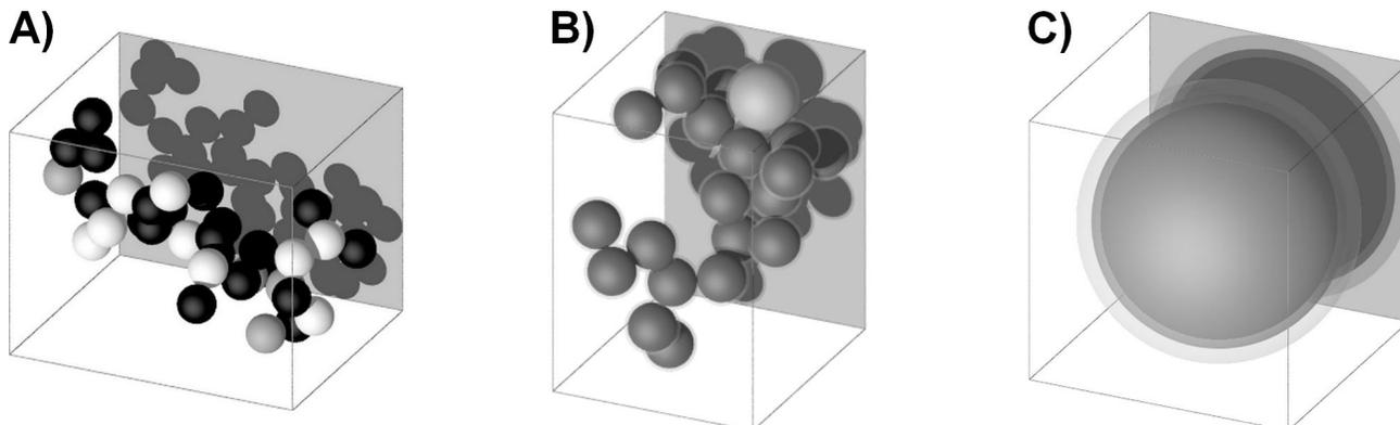
Figure 6. The geometries used for the light scattering simulations: A) The core black carbon aggregate with five spherical sulfate particles and fifteen organic spherical particles. B) The core black carbon aggregate with two ellipsoidal sulfate particles and the organic layer. C) The sphere of equivalent volume.
