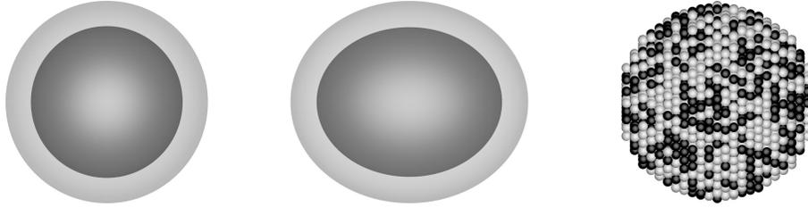
Figure 2: Three geometries used in the first part of the study. They are composed of two materials: black carbon (coloured in black) and organic matter (coloured in gray). Left) A spherical BC particle covered by an external organic layer. Middle) An ellipsoidal BC particle covered by an external organic layer. Right) A spherical particle composed of mixed materials.
