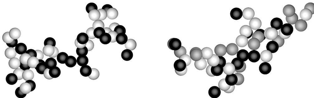
Figure 6: Two fractal-like aggregates composed of  $N_p = 50$  primary particles with the radius  $r_p = 15nm$ . The components are: black carbon (black spheres), sulphate (white spheres) and organic acid (gray spheres).
