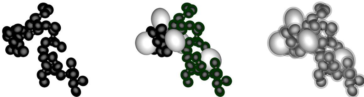
Figure 10: The soot particle used in the study. The core black carbon fractal aggregate (coloured in black) is composed of  $N_{p,c}$  connected ellipsoidal particles. The sulphate particles are coloured in white. The thickness of the coat is  $t_c = 5nm$ .
