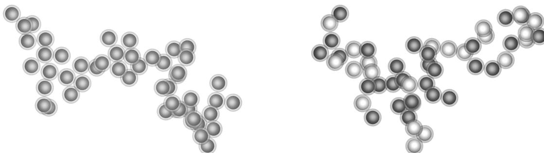
Figure 8: Two fractal-like aggregates composed of coated particles with the radius  $r_p = 20nm$  (including the external layer, i.e.  $t_c = 5nm$ ). Left) Coated black carbon  $N_{p,c} = 50$  particles. Right) Coated black carbon  $N_{p,c} = 25$  and sulphate  $N_{p,s} = 25$  particles.
